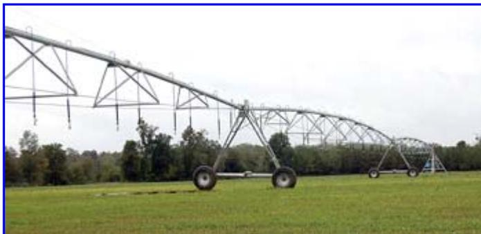
The Bassetts installed this center pivot system that gently sprays water onto the crop using small drop nozzles, causing much less water loss to evaporation and better uptake by the turf grasses.
