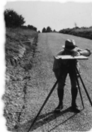
*The early soil scientist used a plane table and sighted through an alidade to plot soil lines on the base map.*
