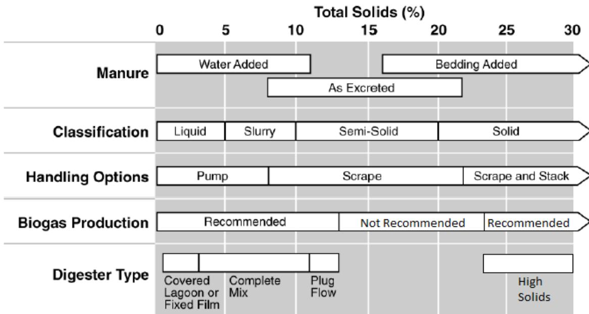
Figure 4. The type of digester selected is affected by multiple parameters and subject to specific design considerations (US EPA – AgStar, modified).
